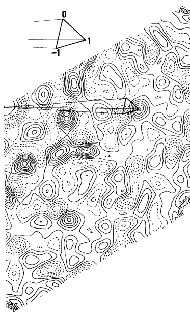
Figure 1. Difference Patterson projection on 0001 within the small P6_3 cell showing the vectors, with weights 1, -1 and 0, between the potassium-vacancy modulation and the O_1 displacements about the triad axis.
